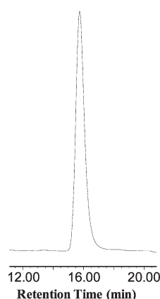
Figure 1. GPC trace of L-PLA produced by ICD/BnOH; M_n = 14.4 kDa, M_w/M_n = 1.12 (run 3, Table 1).
